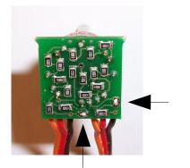
The total resistance of the encoder can be adjusted to your TX by two solder bridges at the rear side of the encoder pcb:
